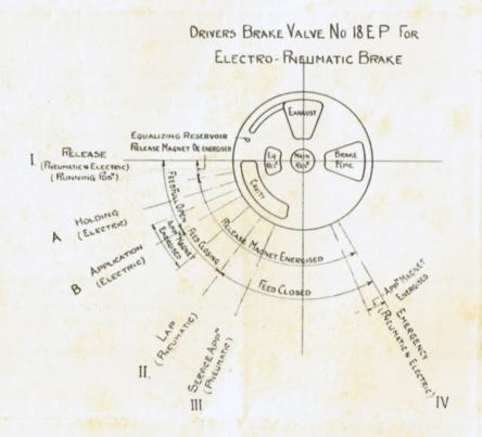
In using the electric control, it will be observed from this diagram that the release magnet is energised and the exhaust of the triple valve is closed from a point between position I and position A up to position IV. Consequently, no matter in what position the triple valve may be, no air can be exhausted from the brake cylinder to the atmosphere, except through the blow-down valve, until the brake valve handle is moved to position I, which is the full release or running position.
