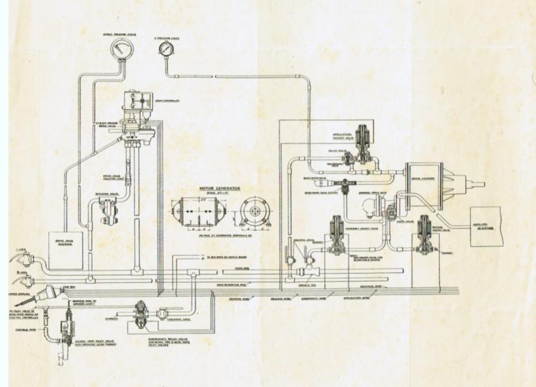
This equipment consists of the Westinghouse Brake Co.'s standard pneumatic brake apparatus, including the improved triple valve giving almost simultaneous action in all applications of the brakes. To meet the demand of certain electric train services, which operate with very frequent stops and require to make shorter schedule time at high speeds, certain electric features have been added, which facilitate the increase and decrease of the pressure in the brake cylinders.
