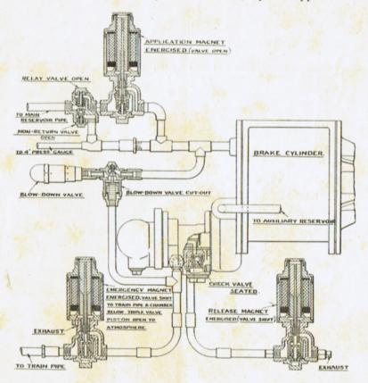
To prevent the pressure in the auxiliary reservoir being increased by air flowing into it from the cylinder when the triple valve is in the application position, a ball check valve is inserted in the regulating plug of the triple valve.
